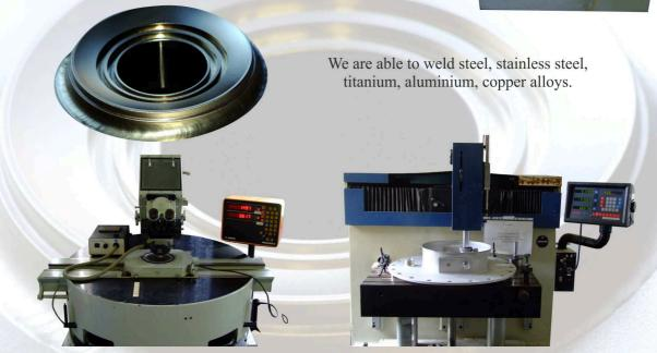
All parts are checked according to ISO 9001:2000 quality standards with profile projector and 3D measuring machine.
